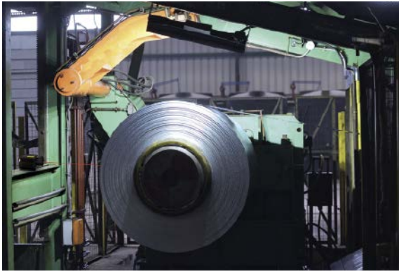
Continuous detection of the coil diameter is necessary in order to monitor the uncoiling process precisely and to determine the changeover time of the coil at an early stage. OptoNCDT ILR2250-100 laser distance sensors from Micro-Epsilon perform this task.
