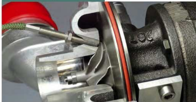
Non-contact turbo speed measurement is possible at levels up to 400,000rpm
