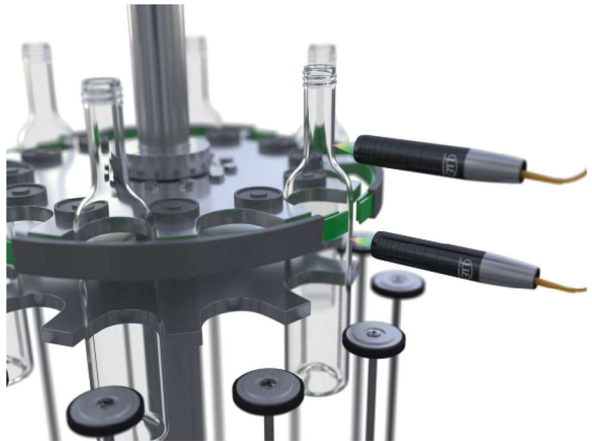
Fig. 1 In container glass production, wall thickness and roundness of the bottles are crucial quality features. This is why these parameters must be 100 % inspected.
