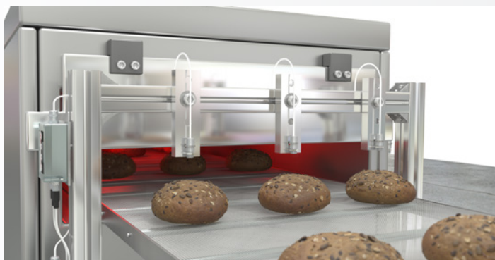
Measuring the temperature of baked goods with thermoMETER UC sensors
