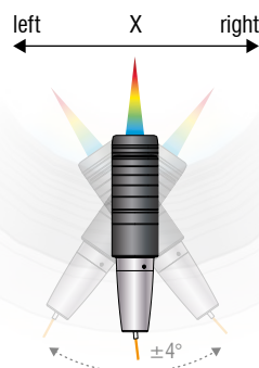
3 Max. tilt angle in X \pm 4^\circ
