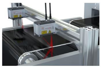
Width, thickness and Heavy Edge of battery film
