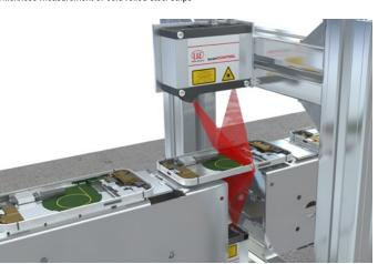
Thickness of smartphone carrier plates
