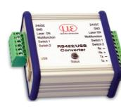
Symmetric differential signals acc. to EIA-422, not electrically isolated from supply voltage. Use a shielded cable with twisted cores e.g. PC1700-x.
