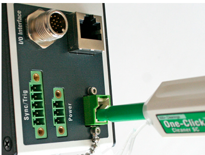
Fig. 10 One-Click™ for cleaning E2000 optical fiber transitions
