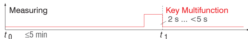
Fig. 65 Flow chart for resetting zeroing/mastering
