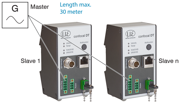
Fig. 29 Synchronization of multiple controllers, star-shaped
