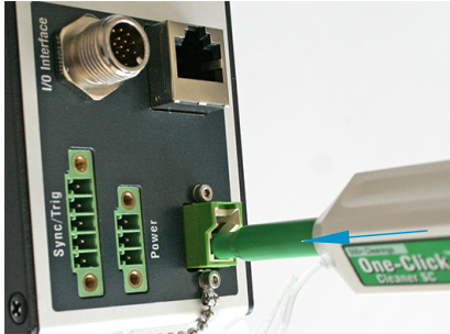
Fig. 82 One-Click™ Cleaner for cleaning E2000 optical fiber transitions
