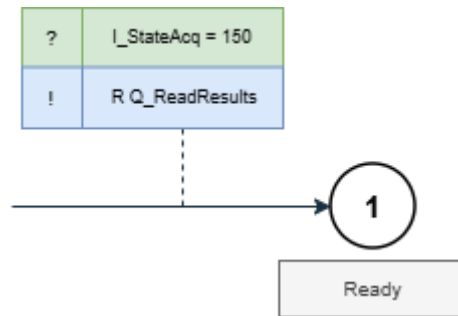
Figure 11: Reset Signal Sequence of the Communication Partner's Evaluation State Machine
