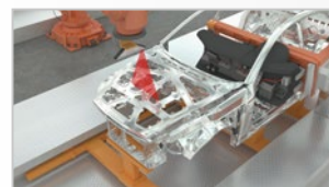
Assembly monitoring in body-in-white production
