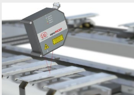
Geometry testing of reflective glass parts
