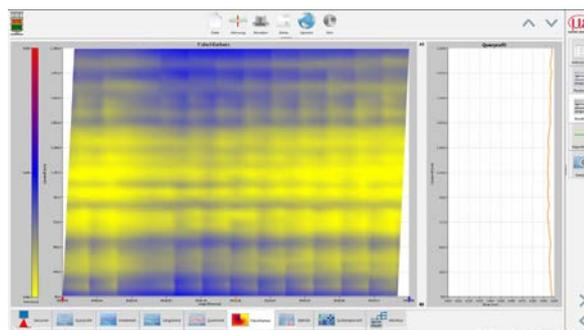
The C-frame includes a multi-touch capable software package for analysis, presentation and archiving of monitored production data. It enables different measurement modes such as fixed track thickness measurement at any position, measurement of the thickness profile, measurement of several longitudinal trends, a SPC package and automated verification of the measurement system's capability.
