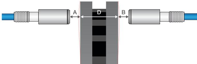
Thickness measurements can be performed in test benches, road tests and in car repair shops using non-contact, capacitive displacement sensors, which detect the thickness of the brake disc from both sides. The thickness is determined by using the difference principle. While the brake disc rotates, the thickness deviation is determined via the circumference of the entire disc. Using several sensors in pairs enables multi-track thickness measurements.
