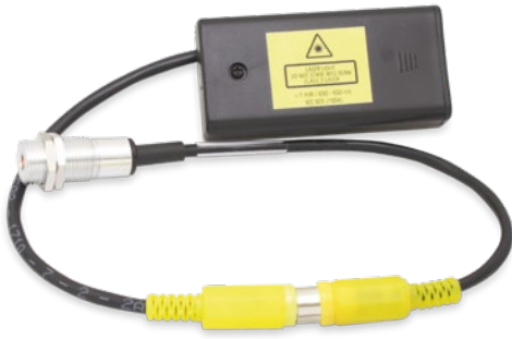
TM-LST-CT Laser sighting aid, battery-operated (2x Alkaline AA), for alignment of CT sensors (dimensions identical to CT sensor)
