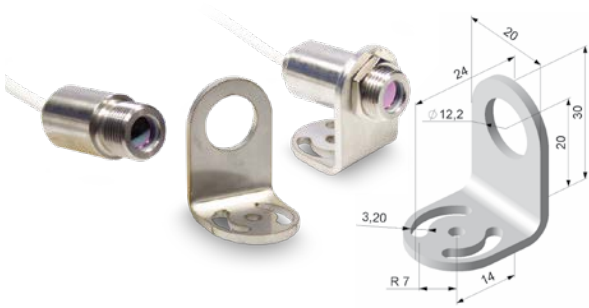
TM-FB-CT Mounting bracket, adjustable in one axis
