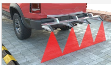
Detection of the road surface profile
