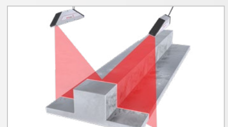
Geometry inspection in metals processing
