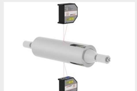
Testing the radial run out of rollers
