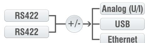
**IF2008/ETH: Interface module for Ethernet connection of up to 8 sensors**
