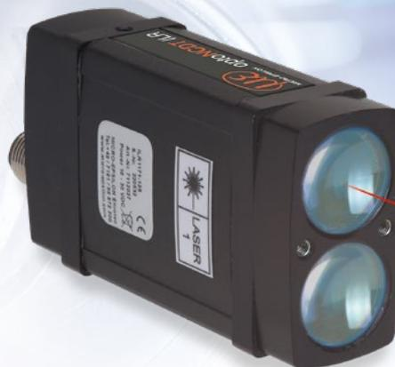
The optoNCDT ILR1171 is a laser-based distance sensor for non-contact and precise distance and displacement measurements from 0.2 m up to 125 m. The measuring range can be extended to 270 m with a reflector film. The sensor is designed for very large measuring ranges, with and without reflector. Due to the very high measuring rate of the sensor, moving objects can be measured easily. Even in poor visibility conditions, the ILR1171 impresses with its high signal intensity for stable measurements.
