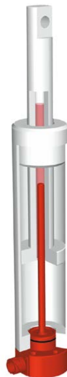
EDS series: integration in a hydraulic cylinder
