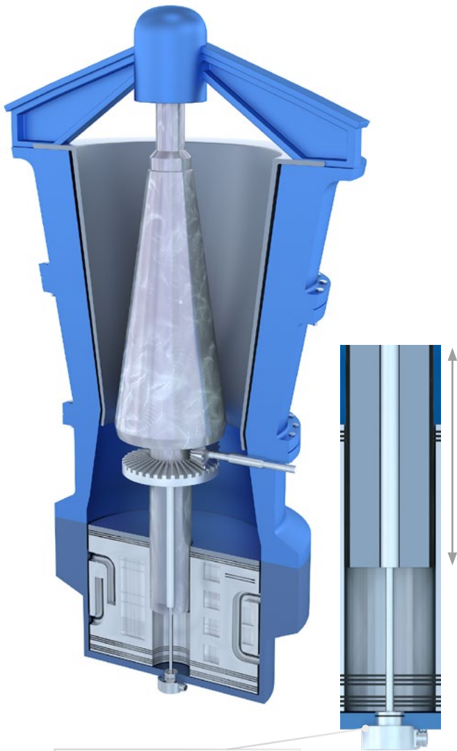
EDS-F: Measuring the grinding gap in crushers
