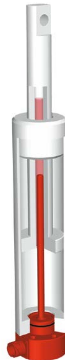
EDS series: integration in a hydraulic cylinder
