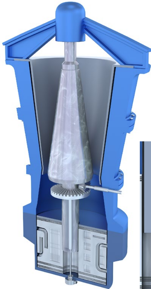
EDS-F: Measuring the grinding gap in crushers
