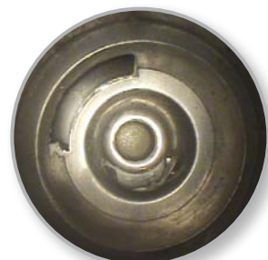
Checking brake cylinder for burrs
