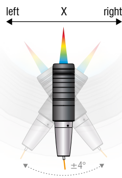
3 Max. tilt angle in X \pm 4^\circ
