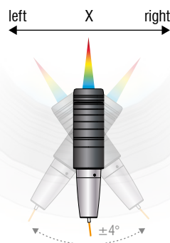
3 Max. tilt angle in X \pm 4^\circ
