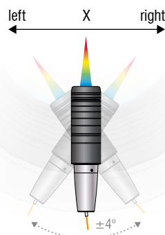
3 Max. tilt angle in X \pm 4^\circ
