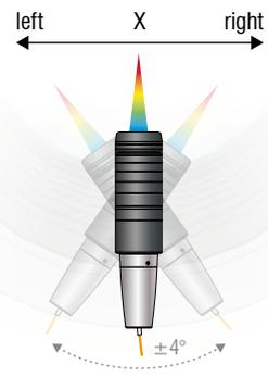
4 Max. tilt angle in Y  $\pm 4^\circ$
