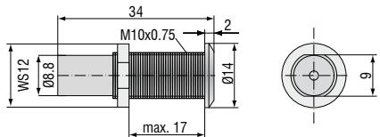
Max. leak rate  $1 \times 10^{-7}$  mbar · l s<sup>-1</sup>, compatible with connector type B
