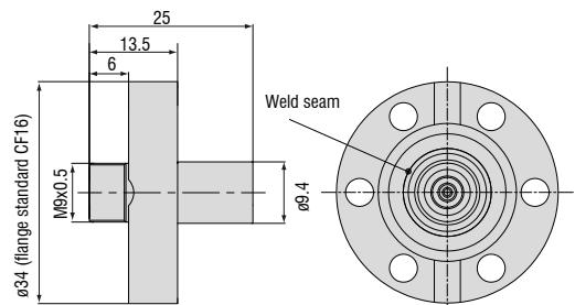
Max. leak rate  $1 \times 10^{-9}$  mbar · l s<sup>-1</sup>, compatible with connector type B
