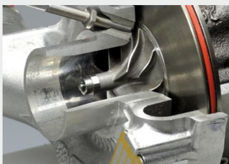
Rotational speed measurement of turbochargers
