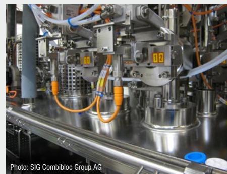
Valve lift measurement in the food industry
