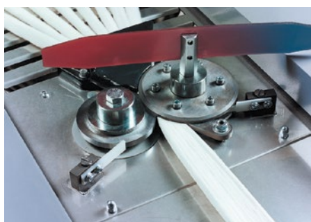
Inline yarn thickness measurement
