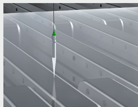
Thickness measurement of flat glass
