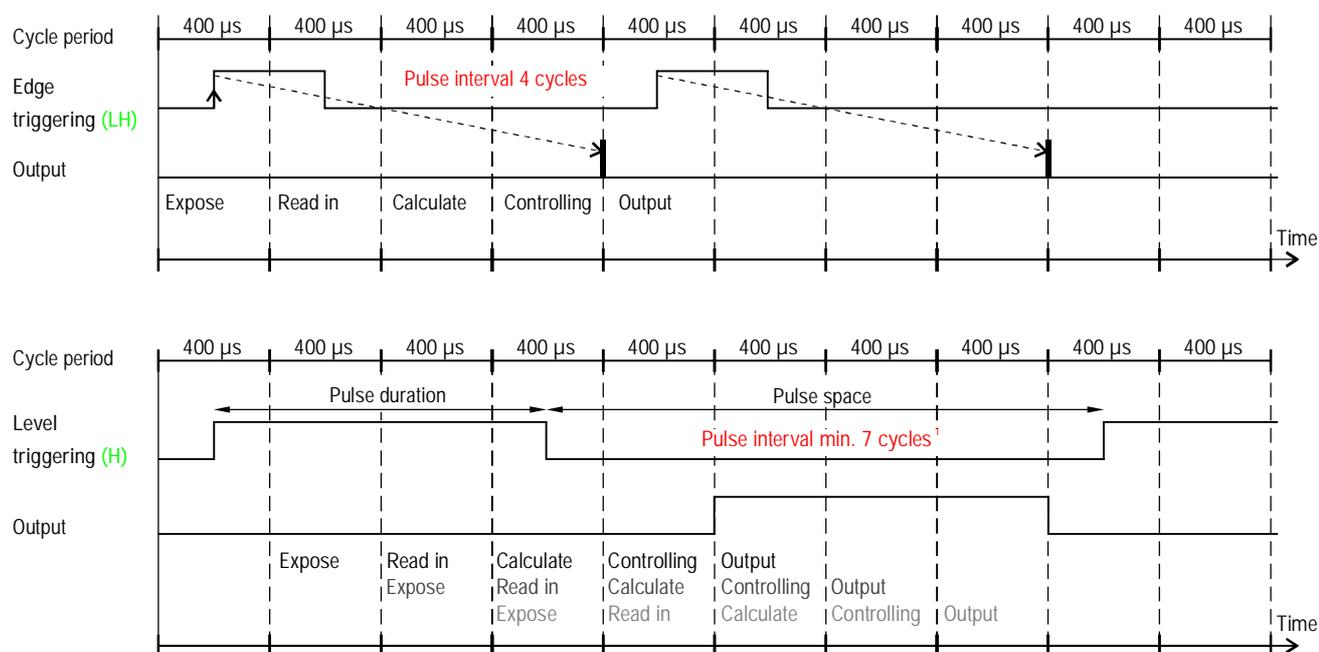
Fig. 4: Time interval with edge (top) and level triggering (bottom), measuring rate = 2.5 kHz
