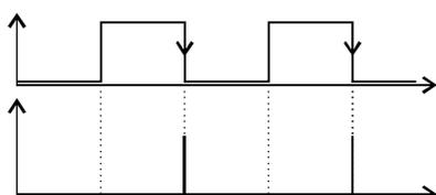
Fig. 1: Falling trigger edge (top) and digital output signal (bottom)
