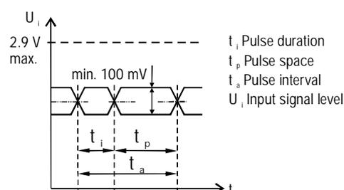
Fig. 3: Trigger signal time characteristics
