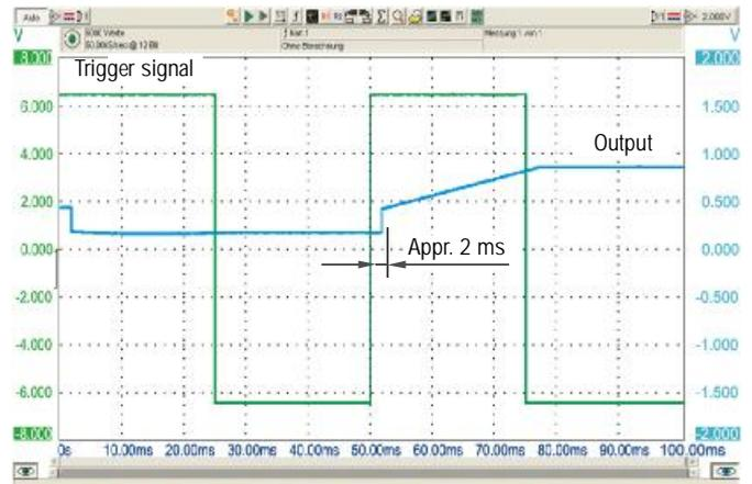
Fig. 5: Time offset between the trigger signal (green, high level) and the analog output signal (blue), measuring rate = 2.5 kHz.
