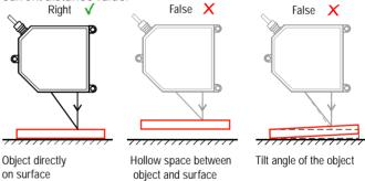
There are high requirements for the support and the conveyor because a hollow space between the support and measurement object or tilting of the measurement object in the measuring gap results in inaccurate measurements.
