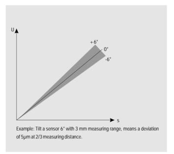
Tilt angles, the controller not linearized for, cause deviations of the measured values in comparison to right angled measurements.
