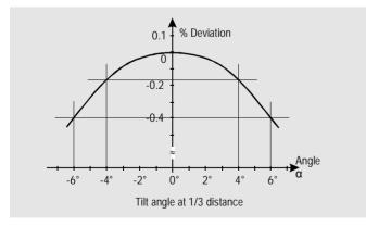
The extent of deviation is different from sensor to sensor. These diagrams were taken with a U6 sensor and aluminium target. The diagrams show, that an inclination of  $\pm 4$  degrees can be accepted and neglected in most applications.
