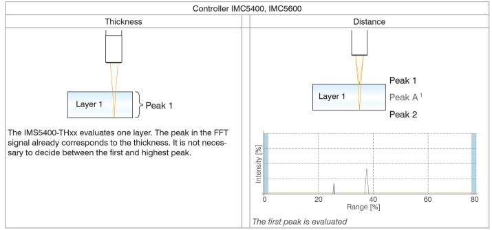
1) During a distance measurement on transparent objects, thickness peaks are displayed in addition to the distance peaks, but the controller does not evaluate them. For the sake of clarity, thickness peaks are marked with letters.
