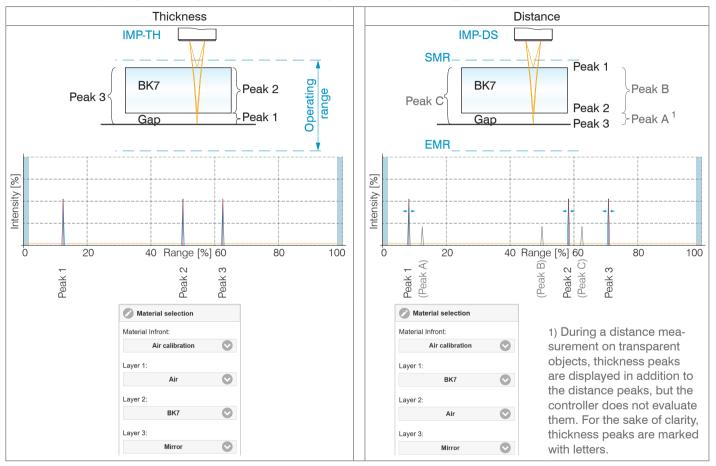
Example of a layer of glass and gap, measpeak sorting: First, corresponding material selection
