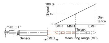
The LED Range on the controller front indicates the position of the target in relation to the sensor.
