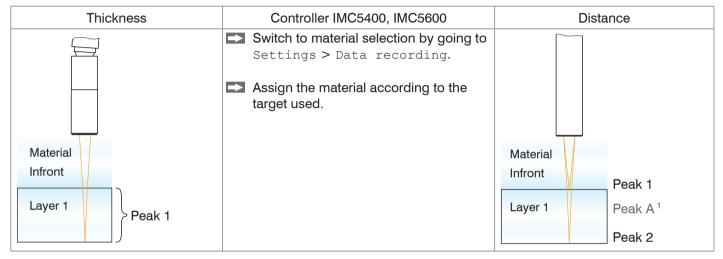
You can edit or add to the material table. For a new material, a phase index and group refractive index is required.
