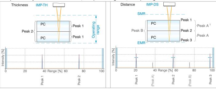
Example of two layers of the same thickness; measpeak sorting: First, corresponding material selection
