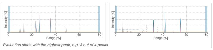
The number of peaks of the FFT signal that are used for evaluation in distance and thickness measurement are to be determined separately, see Chap. Material Selection.
