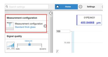
The signal quality is set to Balanced at the factory.
