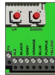
Fig. 10 Opened controller with terminal connections
