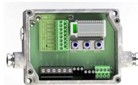
Fig. 10 Opened controller with terminal connections
