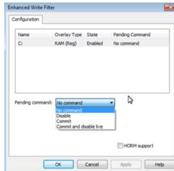
Fig. 34 Screen Write Protection Filter - Pending command 1
