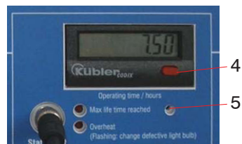
Fig. 75 Operating time counter on the front of the Xenon light source
