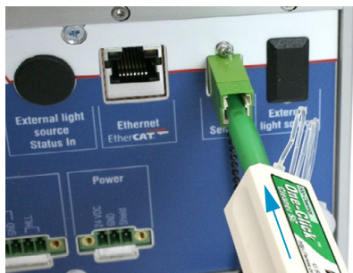
Fig. 82 One-Click™ for cleaning E2000 optical fiber transitions
