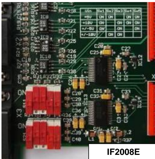
Image 4: Switch settings ADC level (Settling in the image \pm 10 )
