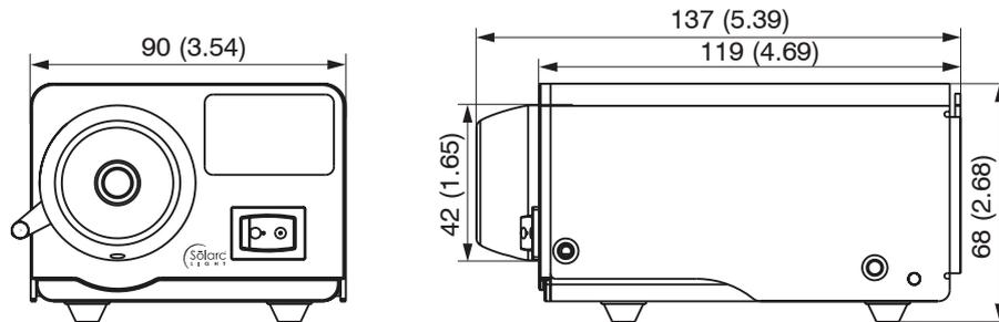
Fig. 1 Endlight FOT Xenon light source – dimensional drawing
