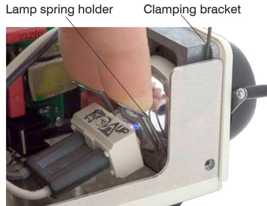
Fig. 12 Press down the lamp spring holder
