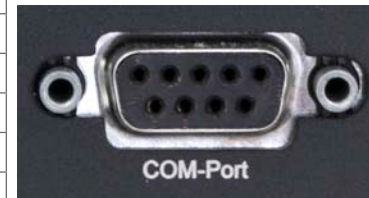
Fig. 11 9-pin. COM-Port female connection respectively RS232 interface
