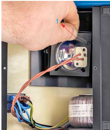
Fig. 10 Lift the spring clip
