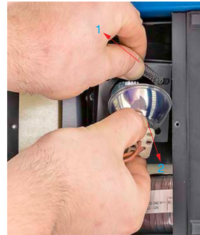
Fig. 11 Loosen the lamp
