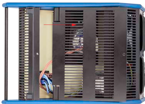
Fig. 8 Remove the bottom cover
