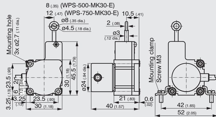
Dimensional drawing of WPS-...-MK30, with incremental encoder, dimensions in mm (inches)
