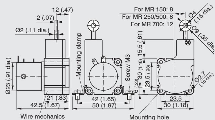
Dimensional drawing of WPS-...-MK30, with potentiometer, dimensions in mm (inches)
