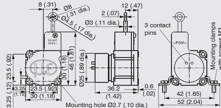
Dimensional drawing of WPS-...-50-MK30, with potentiometer, dimensions in mm (inches)
