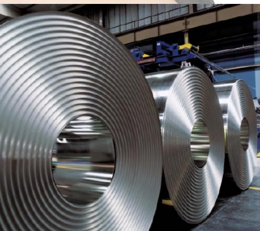
Coils are the raw material for many other products; an important quality criterion of the metal strip is the preferably constant thickness
