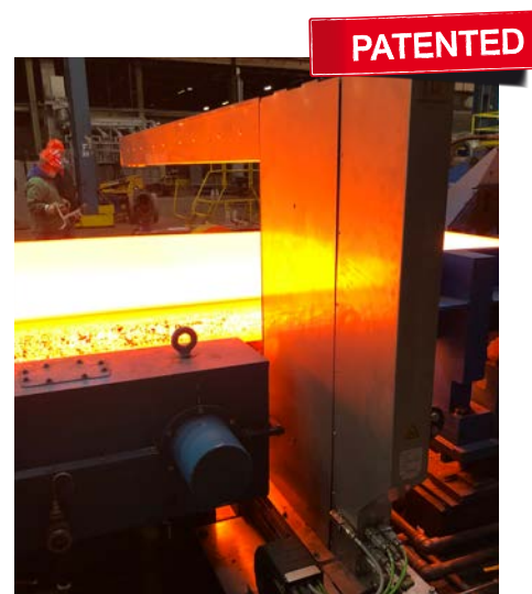
Patented Blue Laser Technology for the measurement of red-hot glowing metals with more than 700 °C
