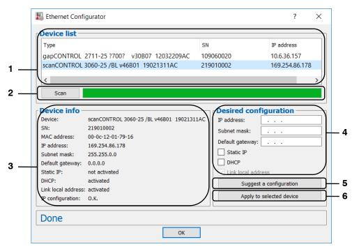
Fig. 3.53: "Ethernet Configurator" dialog box
