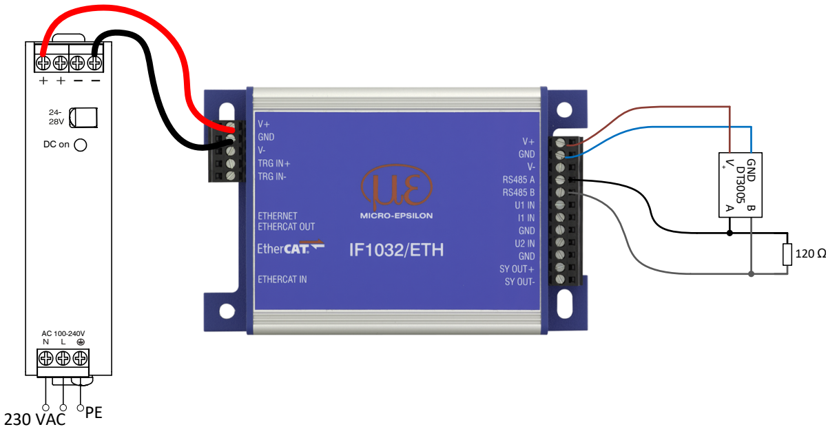
Fig. 21 Connection of the eddyNCDT 3005 controller to the IF1032/ETH interface module with optional PS2020 power supply unit
