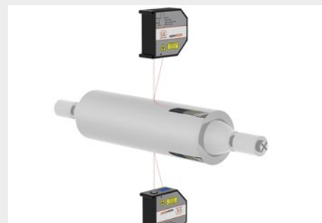
Testing the radial run out of rollers
