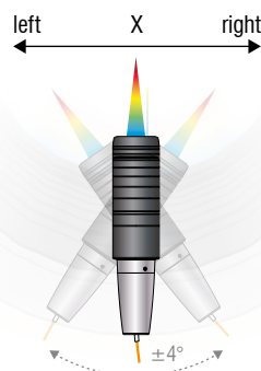
3 Max. tilt angle in X \pm 4^\circ
