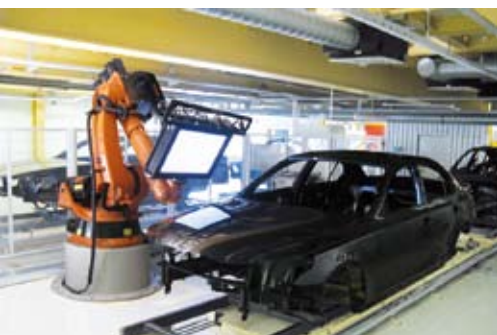
reflectCONTROL Robotic during defect inspection on painted bodyshells
