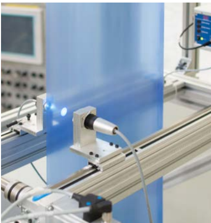
Inline measurement of the color gradient of glass, Plexiglas, PET and PVC foils, paper.
