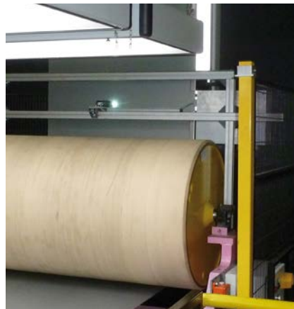
Measurement of the zinc sheet color.
