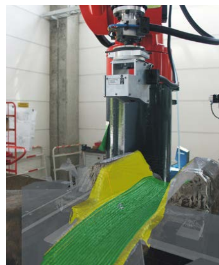
scanCONTROL data (yellow), calculated welding lines (green)
