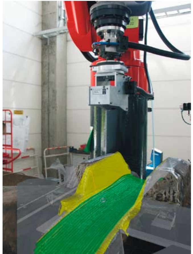
scanCONTROL data (yellow), calculated welding lines (green)
