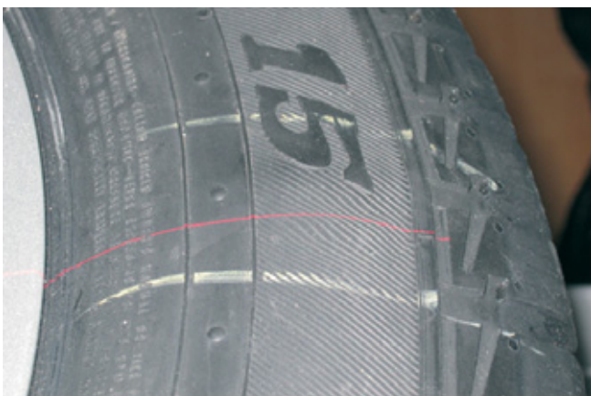
Bulge on the tire - visible on the laser line
